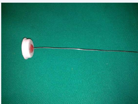
Figure 2 30 Gauge wire attached to the centre of the disc using self-cure acrylic.
