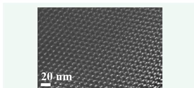
**Figure 1** HRTEM image exhibiting well-ordered structure and uniform array of pores in SBA-15 sample, one of the highly explored materials of porous solids.
