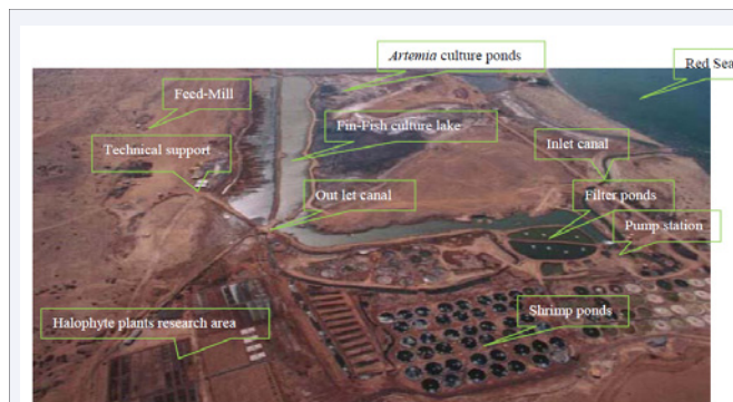
Figure 3 Integrated seawater farm; including inlet-canal, pumping station, physical filter ponds, shrimp ponds, outlet-canal, Salicornia research area, canals (finfish culture), Artemia ponds, technical support, feed-mill and office at Seawater Farms Eritrea (SFE), Massawa, Eritrea. Source: adapted from the 2nd International Symposium on Bio-fuels, March 31, 2010, Delhi, India.
