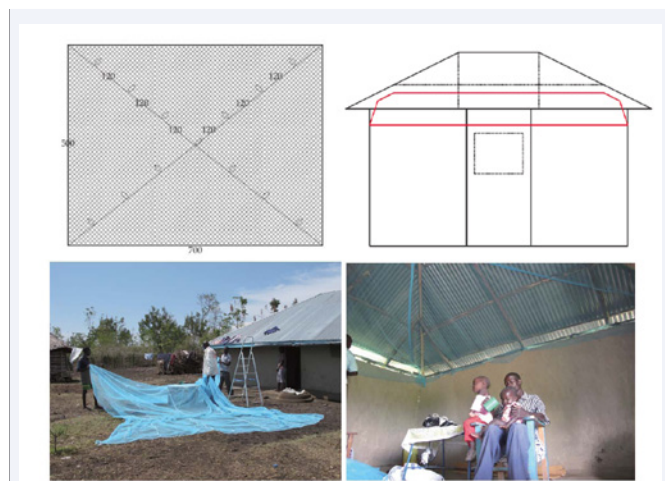
Figure 6 Ceiling net using Olyset® Net materials (upper left) and an outline sketch of the ceiling net installed in a house (upper right). Intervention scene with a ceiling net (bottom left & right). The study was performed in 3 houses in Nyandago village, Gembe East, Mbita Division, Suba district of Nyanza province, western Kenya. Two houses (NYAND 8 and 11) were used as intervention houses, while the third (NYAND 6) constituted a control. One-and-a-half ceiling nets (7 × 5 m plus 3.5 × 5 m) were installed to cover each house. The bottom edges of the ceiling nets were stapled onto the edge of eaves or mud walls, to close the openings of the eaves.
