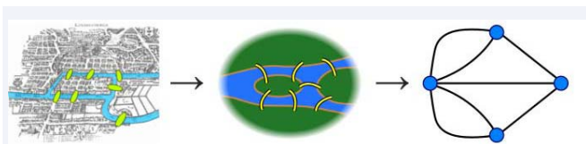
Figure 1 Euler's Königsberg graph theory problem from (Wikipedia contributors. 2016). This theory provides the basis for all network modelling methods used air flow handling, water supply and traffic systems.
