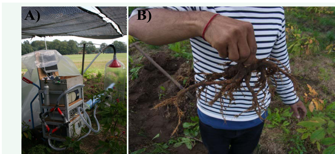
Figure 3 (A) – Portable unit used for ^{13}\text{CO}_2 -labeling of P. ginseng under field conditions (B) – Roots of ^{13}\text{CO}_2 -labeled P. ginseng that yielded the ginsenosides \text{Rg}_1 and \text{Rb}_1 described in this study.
