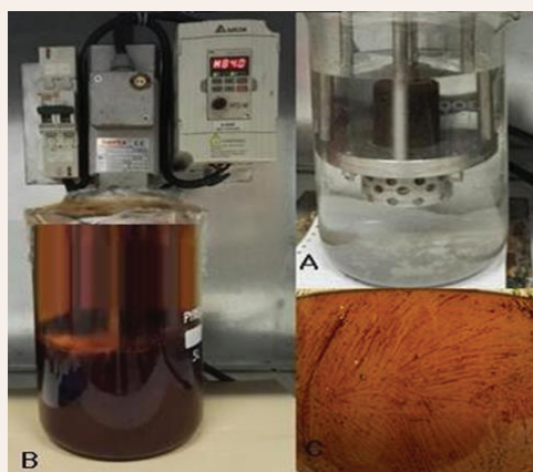
Figure 4 A: Before oxidation stage, B: After oxidation stage, C: flow pattern of shear mixer performance
