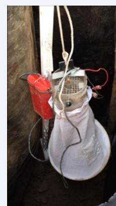
Figure 1 CDC light trap set in a mud-walled house in Marigat.
