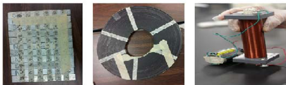
Figure 1 The magnetic field arrangements for the experiment. (a) static field arrangement, (b) Random field generating coil and (c) Electromagnetic field inside the coil which perfectly fits a test tube attached with 3V battery.
