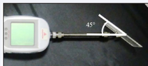
Figure 1 Photograph of a digital force gauge. The image shows the tension jig that was fitted using a hook-shaped component and the acrylic plate attached at a 45° angle.
