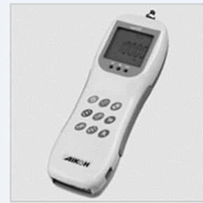
Figure 1 The digital force gauge. Measurements are obtained with the hooked apparatus attached.
