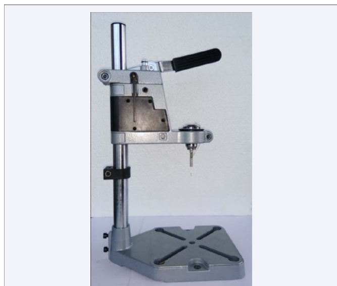
Figure 1b Vertical press stand with attached brass wire in head.
