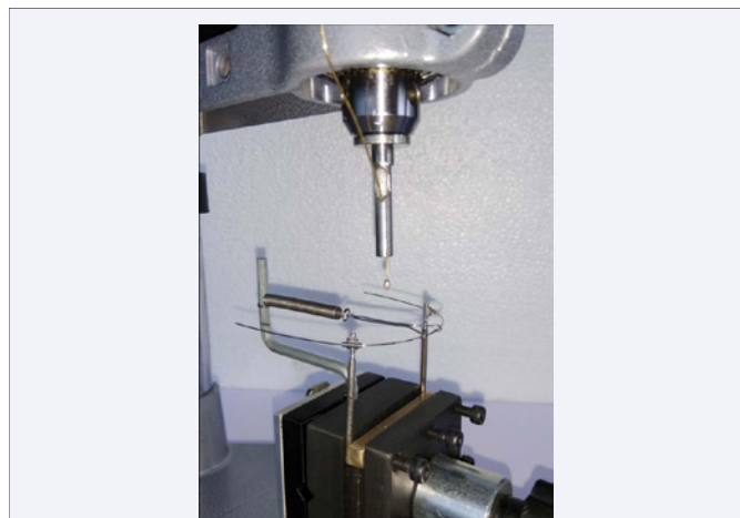
Figure 2a Solder ball on brass wire tip prepared.
