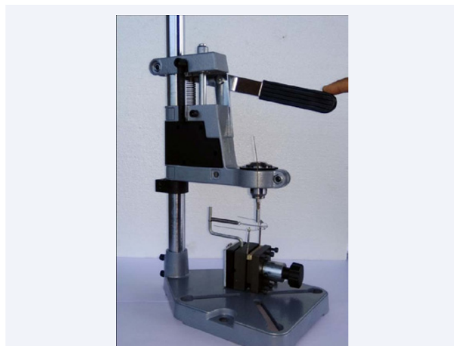
Figure 3b Wires were brought in contact faster just by pressing handle downward.
