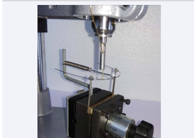
Figure 3a Before soldering, check anticipated contact of vertical brass wire and horizontal archwire at desired marked position.
