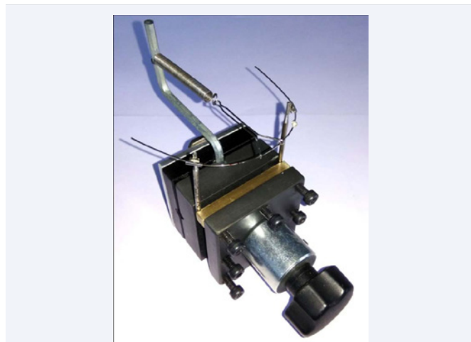
Figure 2b Marked archwire for precisely soldering hooks, inserted in jig.
