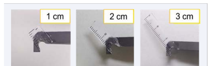
Figure 1 A scale of 1, 2, or 3 cm is attached to each jig at a 45° angle.
