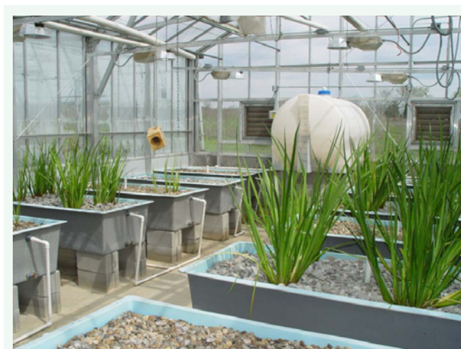
Figure 3 Greenhouse wetland microcosms (n=12) of 182 × 72 × 43 cm each (capacity of 157 gallons) containing two types of bedrocks, crushed limestone and river gravel, and planted with iris plants, Iris versicolor as the plant test.
