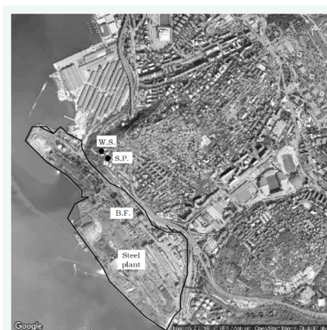
Figure 1 The sampling site in the city of Trieste. S.P.: sampling point for OPC and gravimetric \text{PM}_{10} ; W.S.: weather station; B.F.: blast furnace. The boundary of the steel plant is shown by a black line.
