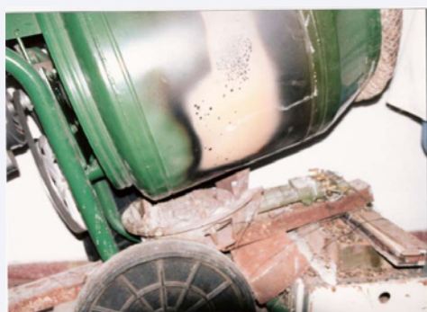
Figure 1 Concrete mixer adapted for the decontamination of sunflower seed hulls as substrate for mushroom cultivation.
