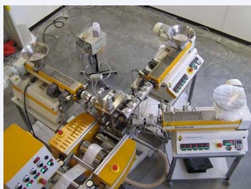
Figure 1 Laboratory set up of Cast film Co-Extrusion.
