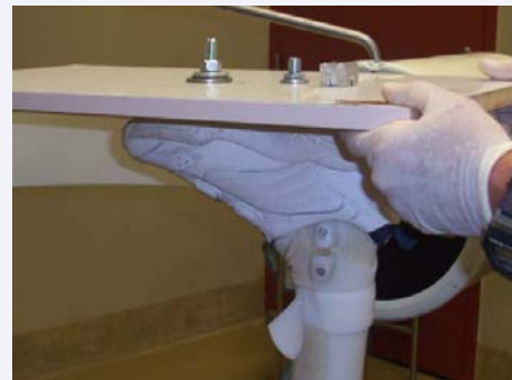
Figure 6 Laboratory Set-up of test platform with AFO/UCBL applied to inverted cadaveric limb and secured to test platform.
