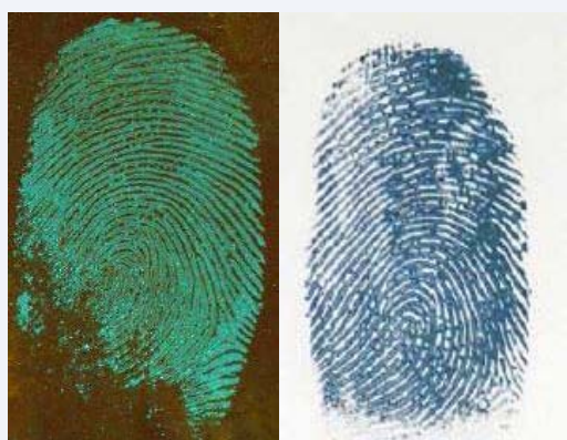
Figure 1 Bloody fingerprints revealed with Acid Yellow 7 (left) and Amido Black (right). Fingerprints are stained yellow after treatment with Acid Yellow 7 and then fluoresce under blue/blue-green light (385-509 nm). Amido Black stains the proteins of blood in a blue-black color. Amido Black can be either methanol or water based as it readily dissolves in both. Images obtained from an exercise made by the Gendarmerie Nationale in Orléans, France.
