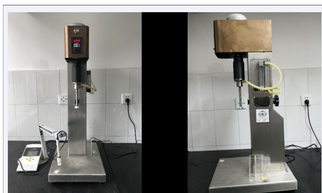
Figure 2 Schematic of XFG-type flotation machine.
