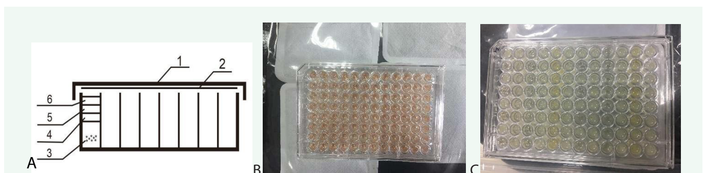
Figure 1 A. Design of microplate device for anaerobic culture, 1 microplate cover, 2 optical film, 3 liquid medium, 4 silicone oil, 5Ve, 6 liquid paraffin ; B. Color of medium before deoxygenation; C. Color after deoxygenation and growth of bacteria
