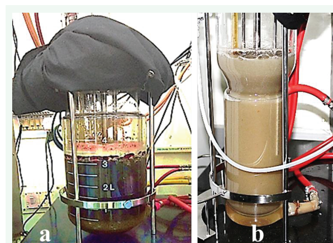
Figure 9 Bioreactor in plant tissue culture a) pigment production in stirred tank and b) biomass accumulation in airlift bioreactor.
