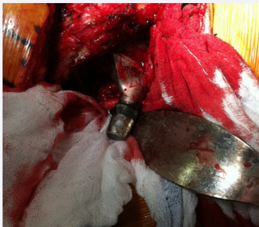
Figure 3 Corrosion present at the junction of the head and trunnion.
