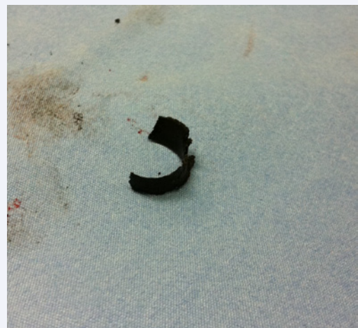
Figure 4 Corrosion after removal from the femoral stem.
