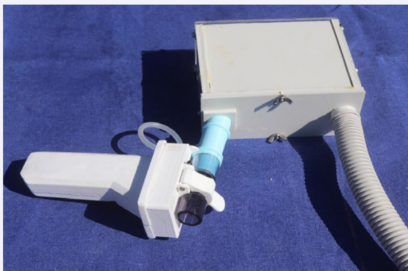
Figure 10 Encased model for rhinomanometric measurement with rhinomanometer 4PR2.
