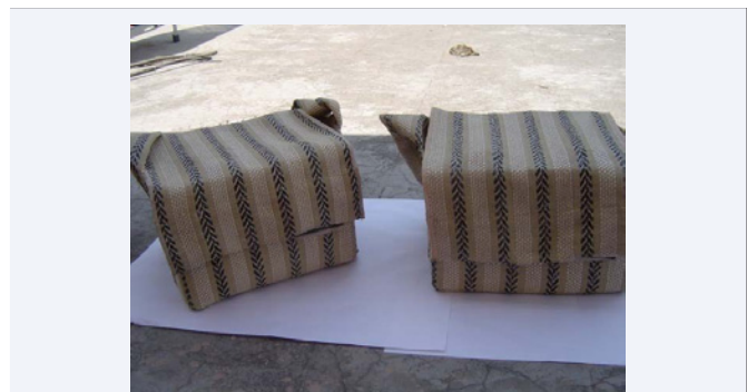
Figure 2 Two Solar Powered Portable Culture Incubators were fabricated. They have cloth covers with shoulder straps.
