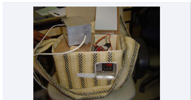
Figure 3 The Solar Powered Portable Culture Incubator can run on AC mains whenever required through an AC battery charger 12 V, especially during the night. The voltage transformer to convert 220 V to 12 V AC is contained in a separate aluminum box.
