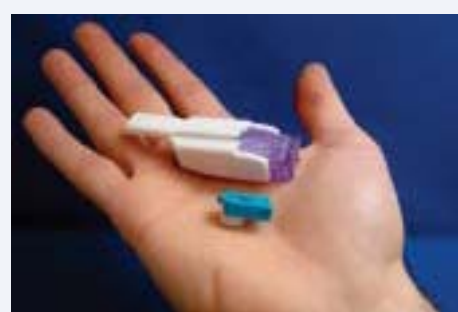
Figure 2 Picture of the Gen2 Technosphere® insulin inhaler device.
