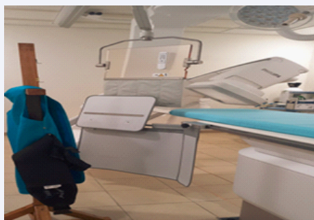
Figure 1 Set up measurement in the Cath-Lab showing staff position for measurements behind the lead shield and lead curtain.
