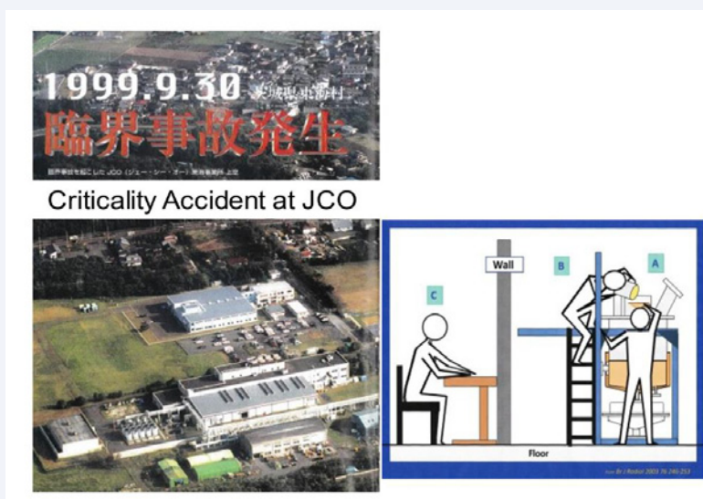
Figure 4 Criticality accident at JCO. Positions of 3 workers when the accident occurred.
