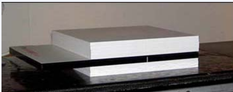
Figure 2 For the field-related verification the 2DARRAY was simply located between RW3 plates. 5 cm RW3 material were below and 4.5 cm above the 2D-Array.
