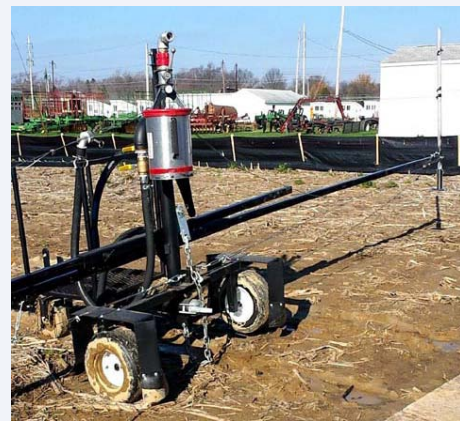
Figure 1 The modified foam depopulation trolley cart, showing the extensions used with the foam generators. The air aspirating foam nozzle was used to aid in foam distribution.
